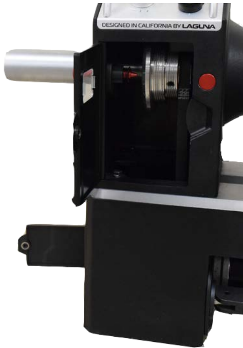
Fig L014 - Changing between speed groups. (1) Low Speed Configuration: 250-850 RPM. (2) Mid Speed Configuration: 430-1450 RPM. (3) High Speed Configuration: 950-3200 RPM. (4) Belt Tension Cam Handle. (5) Drive (Lower) Pulley. (6) 6 Groove Poly-V Belt. (7) Driven (Upper) Pulley.
