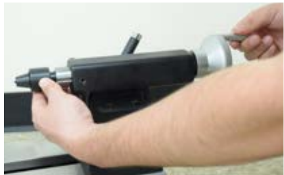
Fig 3.1: Drive center installation
