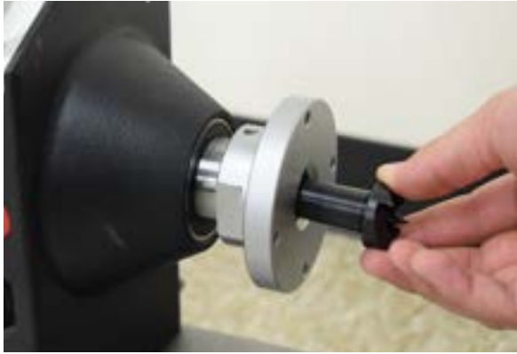
Fig 2: Live center installation
