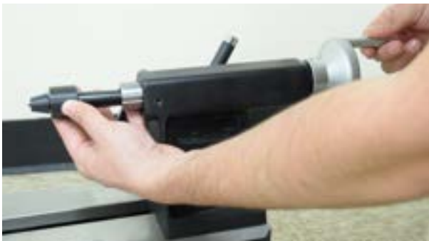
Fig 3: Drive center installation
