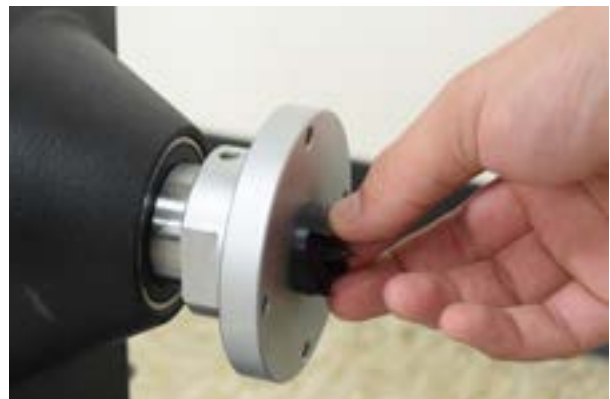
Fig 2.1: Live center installation
