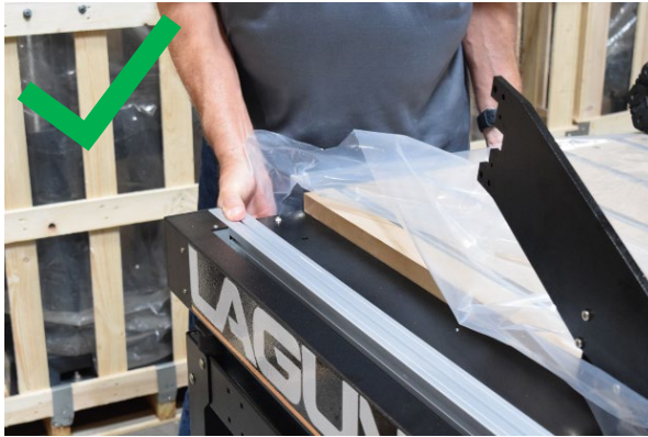
Figure 6-3: Correct Ways to Lift Machine without Forklift
