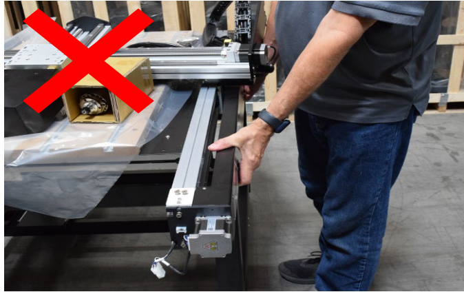
Figure 6-2: Incorrect Way to Lift Machine without Forklift
