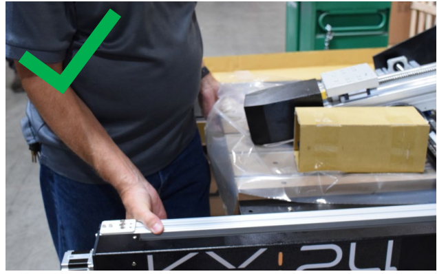
Figure 6-3: Correct Ways to Lift Machine without Forklift
