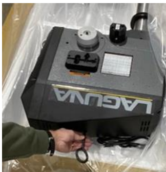
Figure 15: Installing Lifting Eye
