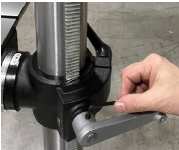
Figures 23-26: Crank assembly
