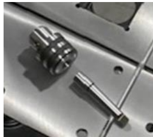
Figure 19: Cleaning Chuck & Arbor
