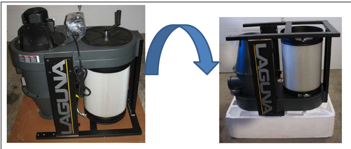
Figure 7: Placing the main component for assembly upside-down
