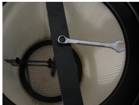
Figure 43: Removing flap pivot bolt (from underneath)
