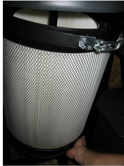
Figures 45-46: Disassembling canister for cleaning
