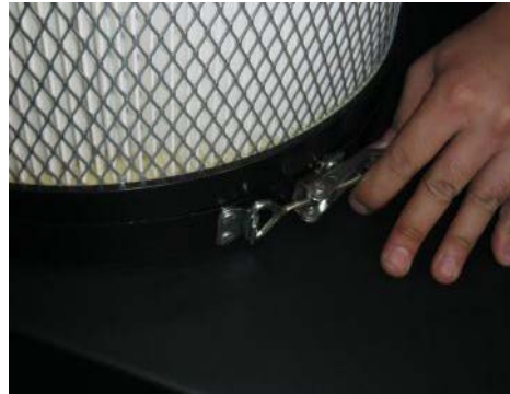
Figure 42: Releasing collection bag clamp
