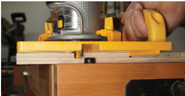
Fig E4 - Setting dovetail cut
